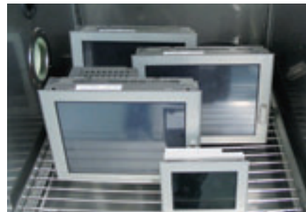
Storage temperature/humidity cycling test
