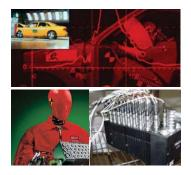
Crash tests in the automotive industrysystem components for short-time data acquisition and processing (measurement boxes) during crash tests in the automotive industry are equipped with ODU MINI-SNAP Push-Pull connectors. Devices for measuring...
