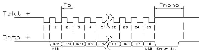
$T_p$  = clock impulse maximum of 2MHz to a minimum of 50kHz. (configured at the cable length setting)
