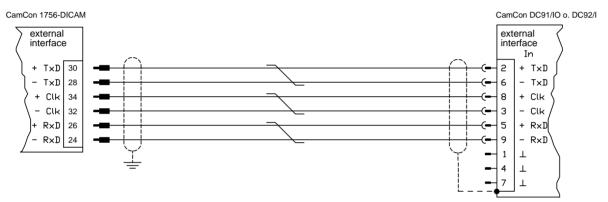
DSUB 9 female plug: Connection for external In- and outputmodules.
