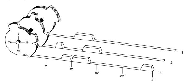
Diagram: Principles of a Cam Switch Unit
