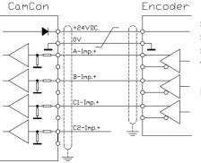
If a 24V PNP signal is used for data input, then only the (+) signals of the inputs may be connected. The (-) signals must stay inactive in this case. The connection of such a measuring system requires a change of the interal switch system and must therefore be stated on the order form.
