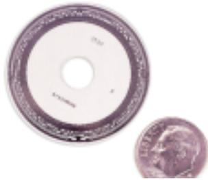
Unlike conventional code disks with a continuous repetition of opaque and transparent fields, the very small CoreTech™ disk condenses absolute position information into one non-repeating circular barcode pattern. A second track with 1024 analog sine/cos cycles is used to enhance resolution and accuracy.
