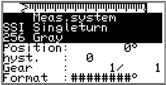
The display gives the resolution of the measuring system in steps per rotation. Generally the CamCon works with a rotation angle coder that has a resolution of 360 steps per rotation. In this case a change in the input value is superfluous. Otherwise the CamCon can be adjusted to the measuring system with the and keys. You can choose between the following predefined resolutions, that are all in accordance with common rotation encoders: 256, 360, 512, 1000, 1024,
