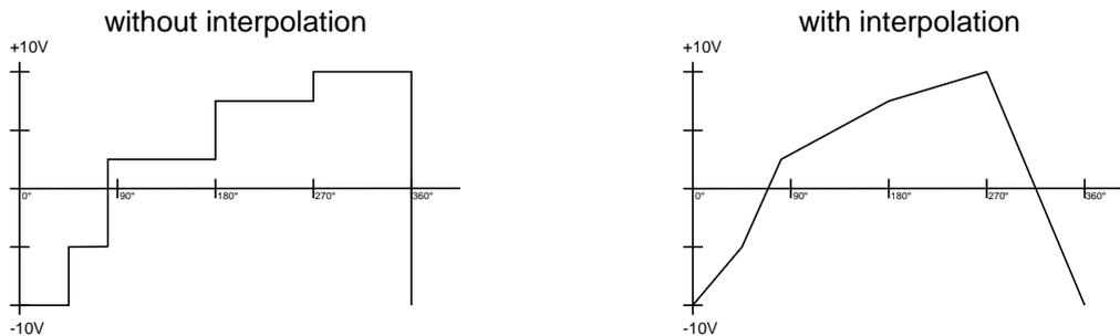
Through interpolation of the definition points, CamCon can adjust the values and present a curve, corresponding to the above right drawing.
