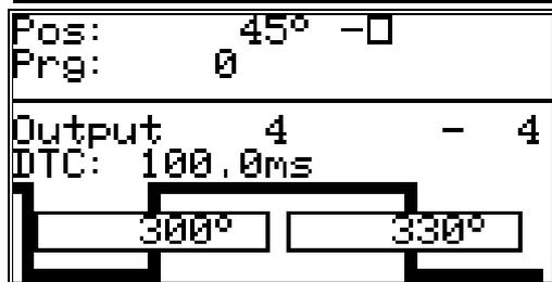
8. Press the **CR** key to confirm your input. The second cam is programmed.
