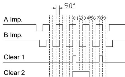
The signals Clear 1 and Clear 2 are a standard AND linked and their function can be changed through the software. See chapter "7.4.1.5.3. Inkremental-measuring system" on page 43
