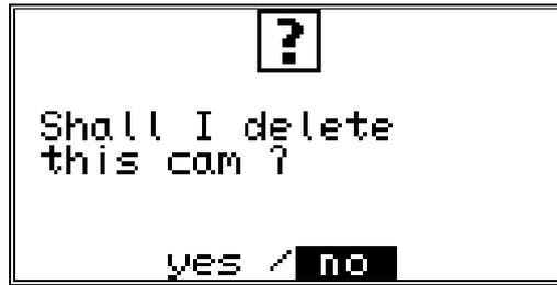
To delete the cam, move the cursor to "yes" with the
