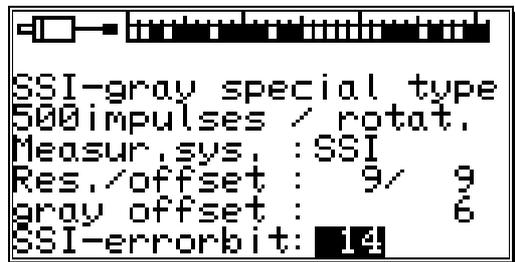
**Attention:** *The position of the data bits can be seen in the graphic in the upper part of the display. You can determine the positions of the LSB, HSB and errorbits quite easily by moving the measuring system.*
