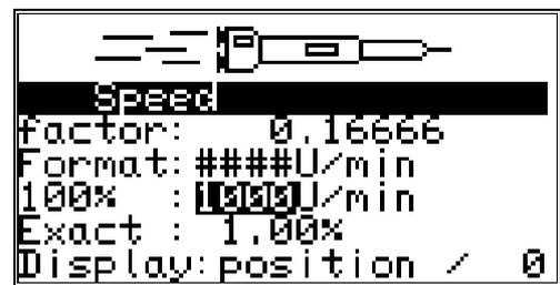
entered value, for 1000 rotations per minute it lies at 50 rotations per minute. Press the key or the key to move the cursor to the next menu point "Exact".
