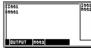
Register 2 is activated for one cycle when the signal at input 1 changes from 0 to 1.
