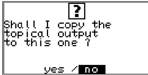
Move the cursor to "yes" with the **←** key and press the **CR** key to confirm your input. This starts the copying process. After a short while the new output will appear on the display.
