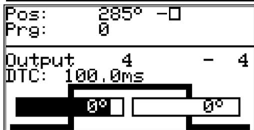
4. Press the **INS** key to enter the cam activation point for an additional cam. The cursor moves to the input field for the cam activation point; a stylized cam starts to blink simultaneously.
