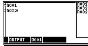
Output 1 of the CamCon is enabled when the rotation direction output 32 is **active**.
