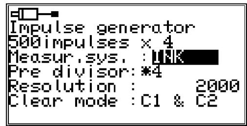
1. Enter the value of the prescaler (predivisor) with the  and  keys. The prescaler divides or multiplies the incoming impulses from the measuring system with the defined value. The following scalars can be entered: "\*4", "\*2", "\*1", "/2", "/4", "/8", "/16", "/32", "/64", "/128", "/256", "/512".
