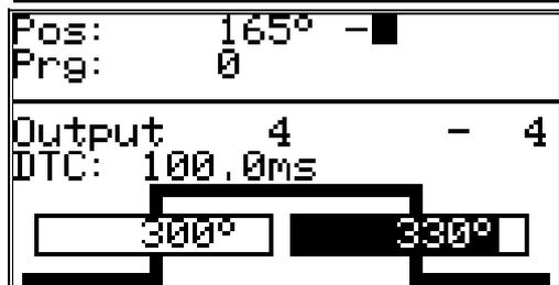
6. Press the **L** or the **CR** key. The cursor moves to the input field for the cam deactivation point.
