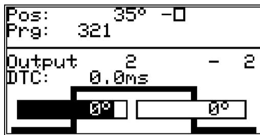
After you confirm your selection with the **CR** key, the field for the cam deactivation point is underlined in black. Simultaneously, the dropping flank of the stylized cam starts to blink.
