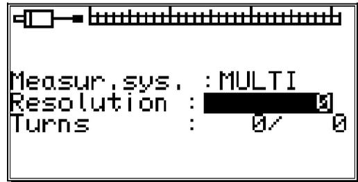
**Example 1:** You have a rotation plate with an electronic gear rate of 3 to 1, i.e. the encoder rotates 3 times for every rotation of the plate. These three rotations correspond with 360 impulses (360 degrees). You need to make the following inputs:
