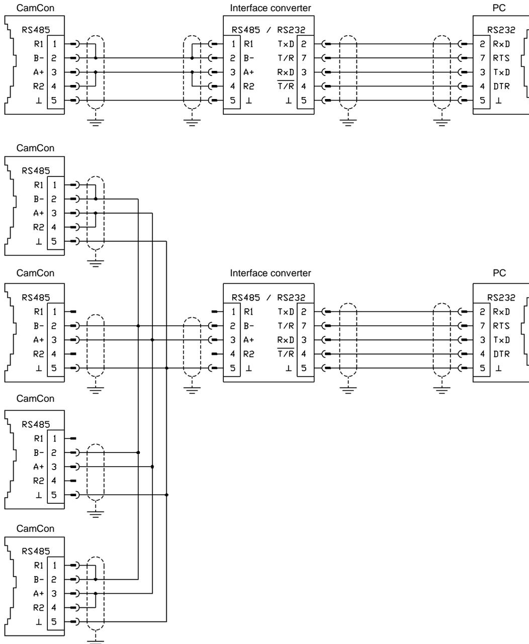
**Please note:** On the first and the last unit in a chain connected via the RS485 interface, pins 1 and 2, as well as pins 3 and 4, of the connection plug have to be bridged to effectively close-down the the data and the reception cable. For this purpose, pins 1 and 4 are equipped with close-down resistors.
