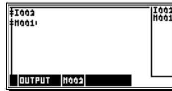
Register 2 is activated for one cycle when the signal at input 2 changes from 0 to 1.
