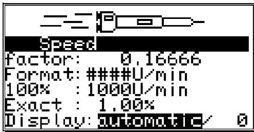
If you want to prevent the automatic switching at the 5% of the maximum speed in the "Display" menu point, you can select one of the three different display types with the  key and the  key.
