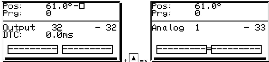
The output numbers of the analog cam outputs are always added to the numbers of "normal" outputs and this number can be selected directly from the programming menu. If you have configured e.g. 32 cam outputs, the number of the first analog cam starts at the output 33. The output number of the analog cam changes automatically when you change the number of "normal" outputs (see chapter "7.4.6.2. Setting the outputs" on page 55).
