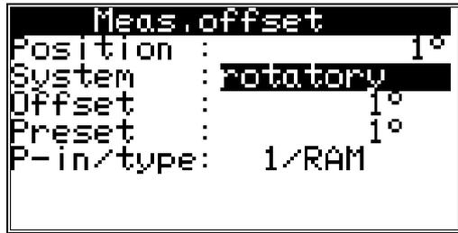
Here you can indicate, using the and keys, whether your controlling system is a rotatory (e.g. an eccentric press) or a linear (e.g. a knee lever press) moved system.
