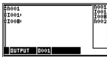
Output 1 of the CamCon is cleared if inputs 1 and 8 are active.
