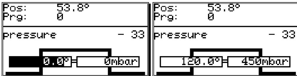
**Note:** As long as only one cam is programmed on a cam track, the programmed analog value is emitted for the whole way of the measuring system.
