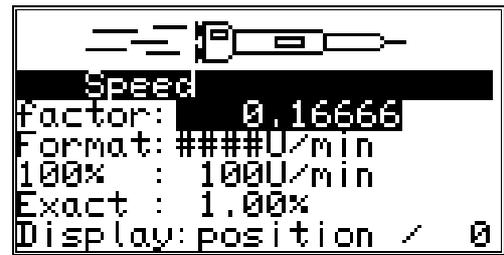
**Example 1:** A rotation encoder with 512 steps supplies 512 increments per minute, which means that the gear runs with 1 rotation per minute. The CamCon measures  $512/60 = 8,533$  increments per second. To receive a display in rotations per minute enter the factor  $1/8,533 = 0,1172$ .
