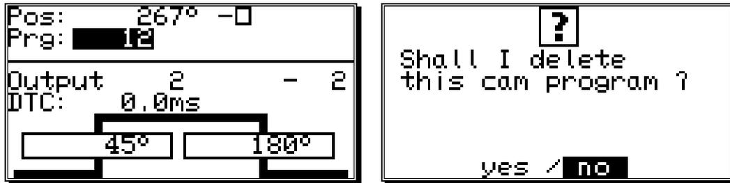
Enter the number of the program that you want to delete with the numeric keys. Press **DEL** and the display shows the security precaution question for the deletion of programs. Move the cursor to "yes" with the **◀** key, and press the **CR** key to delete the program.
