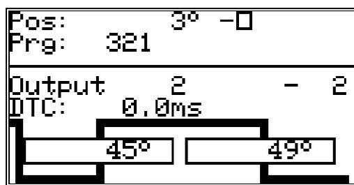
The increasing course of the cam curvature on the right edge of the display points to another cam that is positioned between the cam deactivation point (180°) and the higher border of the measurement range (e.g.:359°). The left flank hints to the presence of additional cams between the cam activation point (45°) and the lower border of the measurement range (e.g.:0°).
