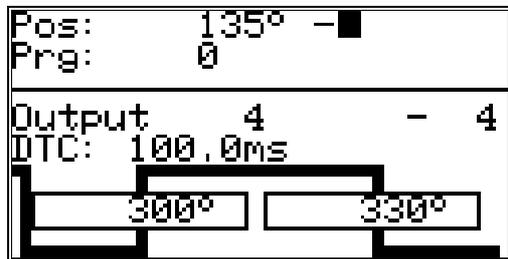
4. Select the inserted cam with the **▶** key.
