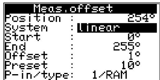
**Attention:** If the range between start value and end value is under- or overshoot during the way gathering of the measuring system, the CamCon switches off with the error message "Pos.Err 3".
