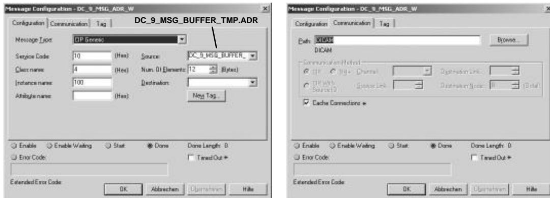
The construction of the source range, in the example "DC\_9\_MSG\_BUFFER\_TMP", consists of 3 DINTs, whereby the first DINT covers the target range (1..255), the second DINT the Offset in the target range (0..255) and the third DINT the number of DINTs which are to be written.
