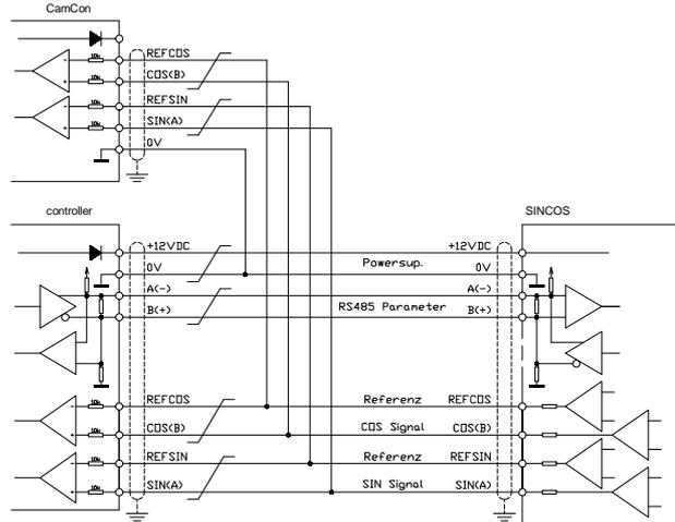
**Note:** The maximum number of revolutions per minute is  $3000 \text{ min}^{-1}$  with 512 Impulse per revolution.
