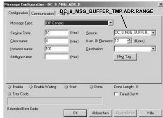
The message can only be set when the bit "CMD\_IN\_USE" (see Chapter "4.13.2. Status Bits in the I - Range") is not active. The "DN" bit of the message itself as well as the bits "CMD\_OK" or, in the case of an error the bit "CMD\_ERROR", confirm this MSG. At the end of writing the first message the EXOR\_BIT toggles its place and the "CMD\_IN\_USE" Bit goes back to 0. If the MSG was successful, then the actual data range with the status, the parameters i.e. cams or delay times can be read.
