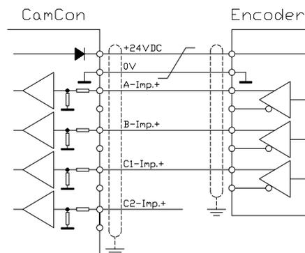
If a 24V PNP signal is used for data input, then only the (+) signals of the inputs may be connected. The (-) signals must stay inactive in this case. The connection of such a measuring system requires a change of the internal switch system and must therefore be stated on the order form.
