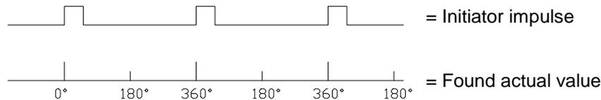
The Initiator can be connected to any free input of the CamCon.
