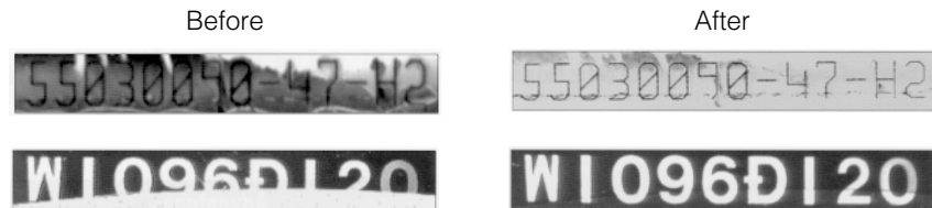
Figure 10. Examples of image improvement with dynamic light control
