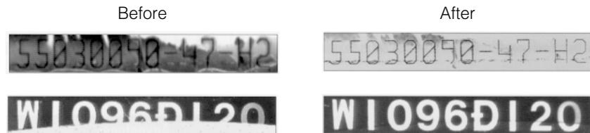
Figure 11. Examples of image improvement with dynamic light control
