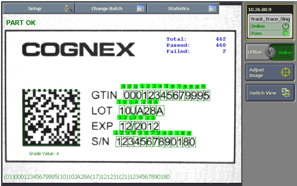
Figure 1-1: Example Track & Trace Run Time Display
