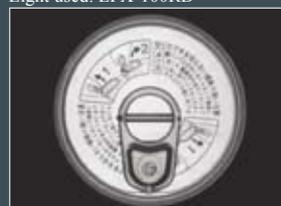
With the LFX at distance of 295 mm from the light to the object, the more collimated light shows the smaller ridges in the can surface clearly.
